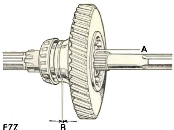
Fig. 10. Checking end-float of the 'low' transfer gear wheel
