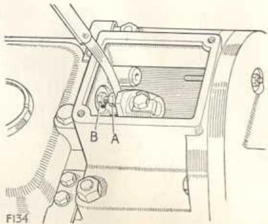
Fig. 14. Adjusting 2nd gear stop bolt
