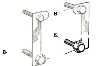
**Fig. 24. Assembling securing bolts to lock-plate**
