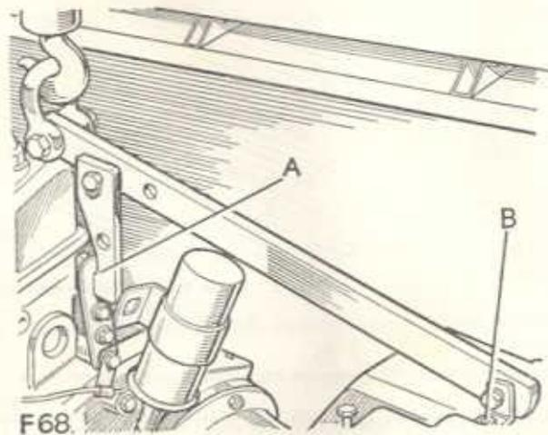
Fig. 5. Engine lifting sling in position
