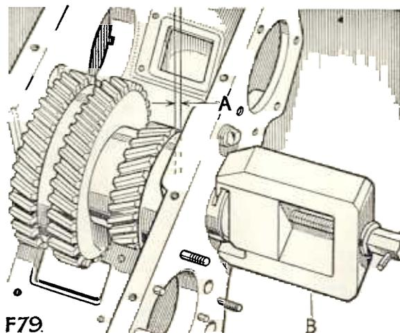
Fig. 8. Removing the intermediate shaft
