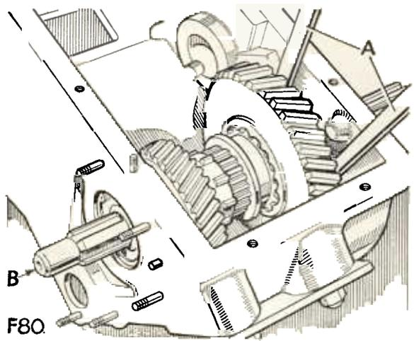
**Fig. 9. Removing transfer box output shaft**
