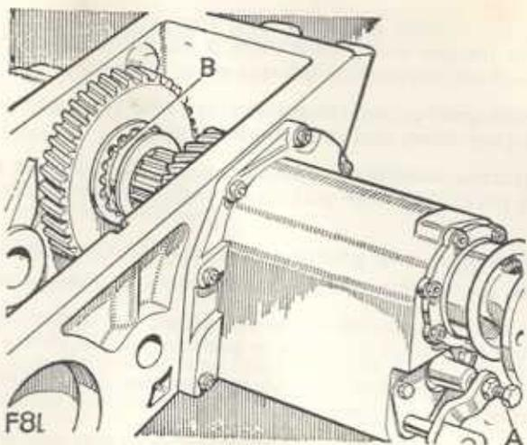
Fig. 13. Setting the transfer selector travel stop.
