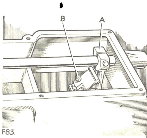
Fig. 20. Adjusting reverse stop hinge plate
