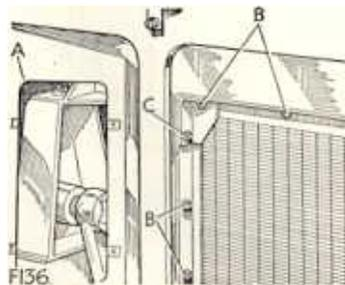
Fig. 25. Radiator securing bolts
