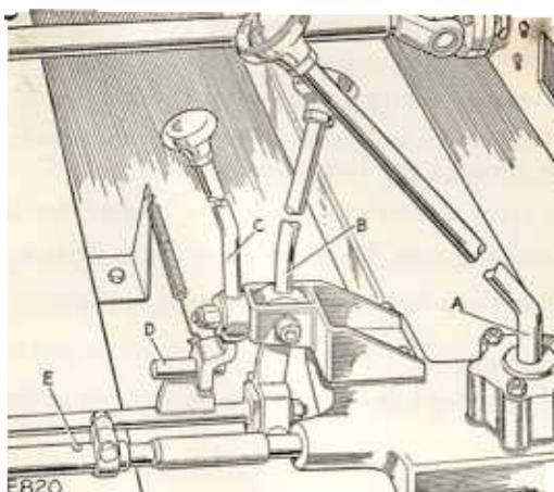
Fig. 21. Setting gearbox control levers
