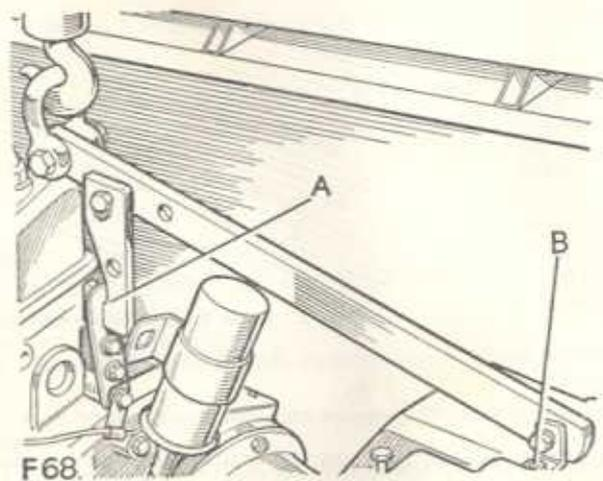
Fig. 5. Engine lifting sling in position
