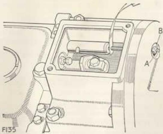
Fig. 15. Adjusting reverse gear stop bolt
