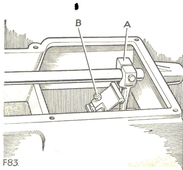
Fig. 20. Adjusting reverse stop hinge plate
