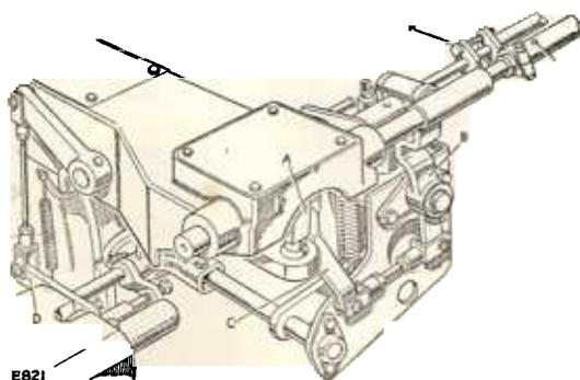
Fig. 22. Setting gearbox control linkage
