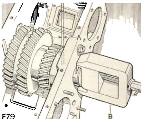
Fig. 12. Checking end-float of intermediate gears
