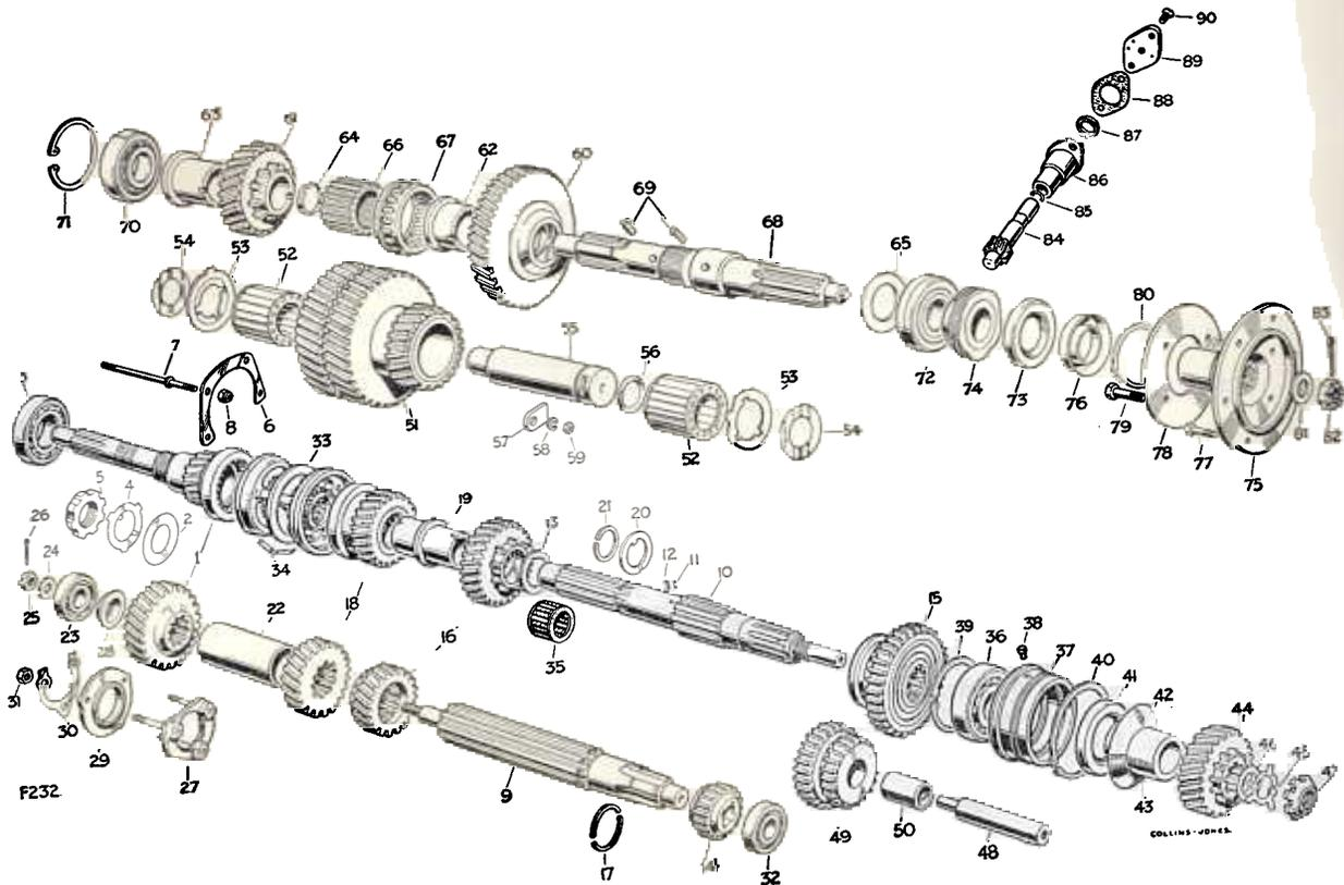
Fig. 6. Main and transfer gear assemblies
